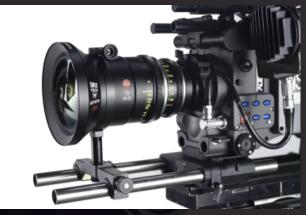
Scorpio Wide Angle Converter Lens keeps the original quality and characteristics of the lenses converted with a conversion of 0.8 approx., a smart combination of exotic glasses that maintains same look and chromatics from the original lens respecting the stop.
